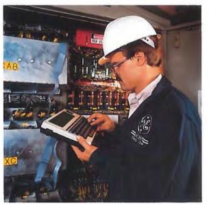
Operational data is transferred from locomotive computer memory to serve engineer's records.
